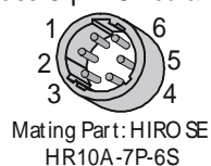
Figure 8: Hirose 6-pin Circular Male—Power Connector
