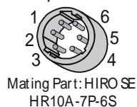
Figure 10: Hirose 6-pin Circular Male—Power Connector
